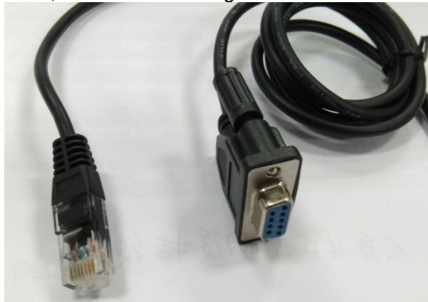
In order to connect these two cables to switch's console port and use the CLI, please connect one of the Male RS232 connector to the Female RS232 connector, as shown in the figure down below:
